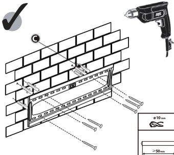
When selecting the position of the TV mount, ensuring that the mount will be mounted on to a flat surface and is level. Mark the wall where the fixing locations are. Drill the holes using a 10mm masonry bit. Using a hammer knock the the wall plugs (C) provided into the wall. Holding the TV mount start in the one corner screw the provided screws (B) into the wall fixing the opposite corners until the mount is secure onto the wall. Ensure all are tight and secure.
