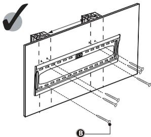
Using the provided self tapping screws (B) type. Holding the TV mount starting in the one corner, screw the provided screws (B) into a wooden joist fixing the opposite corners, until the mount is secure onto the wall. Ensure all are tight and secure.
