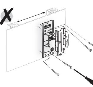
Ensure that the mount is fixed to a solid object and not into plasterboard on its own.
