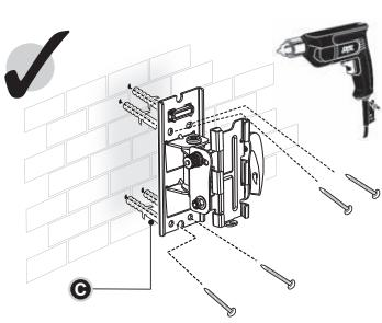
When selecting the position of the TV mount, ensuring that the mount will be mounted on to a flat surface and is level. Mark the wall where the fixing locations are. Drill the holes using a 10mm masonry bit. Using a hammer knock the wall plugs (C) provided into the wall. Holding the TV mount start in the one corner screw the provided screws (B) into the wall fixing the opposite corners until the mount is secure onto the wall. Ensure all are tight and secure.
