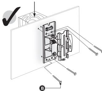
Using the provided self taping screws (B) type. Holding the TV mount starting in the one corner, screw the provided screws (B) into a wooden joist fixing the opposite corners, until the mount is secure onto the wall. Ensure all are tight and secure.
