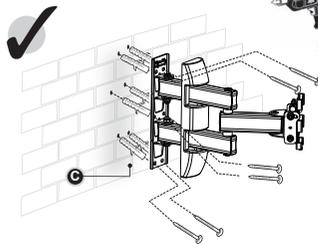
When selecting the position of the TV mount, ensuring that the mount will be mounted on to a flat surface and is level. Mark the wall where the fixing locations are. Drill the holes using a 10mm masonry bit. Using a hammer knock the the wall plugs (C) provided into the wall. Holding the TV mount start in the one corner screw the provided screws (B) into the wall fixing the opposite corners until the mount is secure onto the wall. Ensure all are tight and secure.
