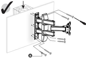
Using the provided self tapping screws (B) type. Holding the TV mount starting in the one corner, screw the provided screws (B) into a wooden joist fixing the opposite corners, until the mount is secure onto the wall. Ensure all are tight and secure.
